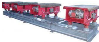
Fig. 1. Appearance of the platform-vibrator with shock that widely used in the construction industry for compaction and molding large concrete products
